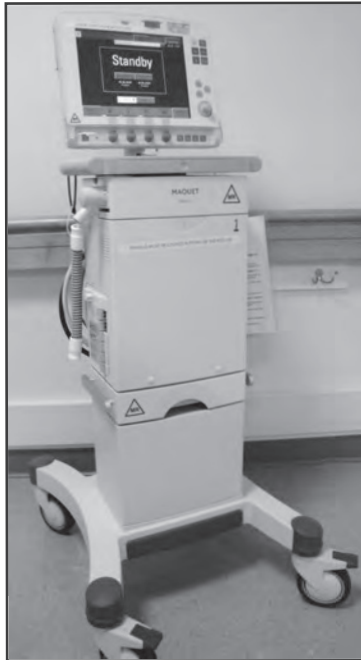
Figure 6. Example of MR Conditional ventilator system (SERVO-i, Maquet Inc., Wayne, NJ). This system includes the ventilator, mobile cart, and battery packs.
