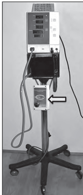
Figure 7. Example of MR Conditional ventilator system. This equipment includes a magnetic field strength alarm system (arrow) (GaussAlert, Kopp Development Inc., Jensen Beach, FL) that is designed to help keep MR Conditional equipment outside of a particular MRI exclusion zone (e.g., 300-gauss).
