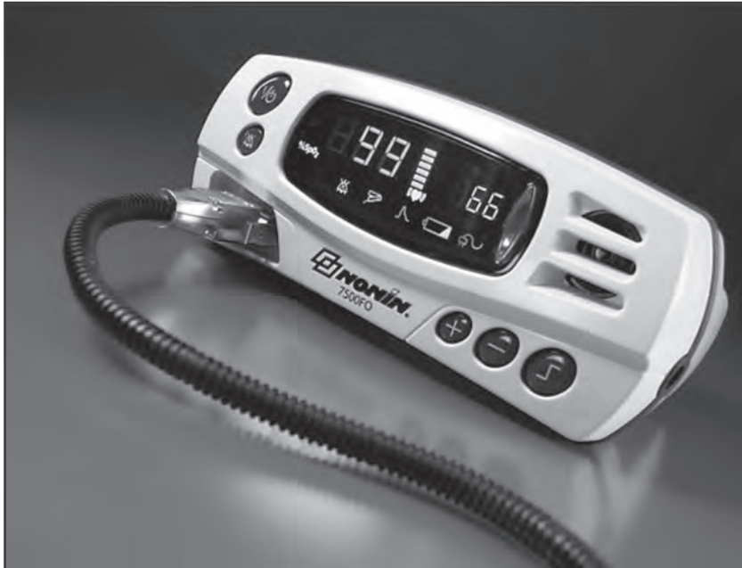
Figure 3. Example of MR Conditional pulse oximeter used to record oxygen saturation and heart rate (Nonin Medical, Inc.).
