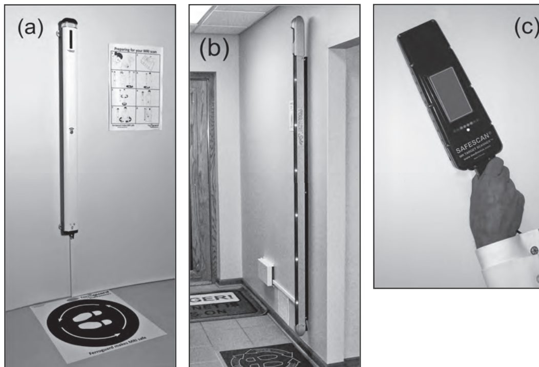
Figure 10. (a) and (b) Examples of wall-mounted ferromagnetic detection systems where patients are screened by rotating in front of these devices. (c) Handheld FMDS that is swept over the patient's body. (Photographs provided courtesy of Metrasens Ltd., Kopp Development Inc., and Mednovus, Inc.)
