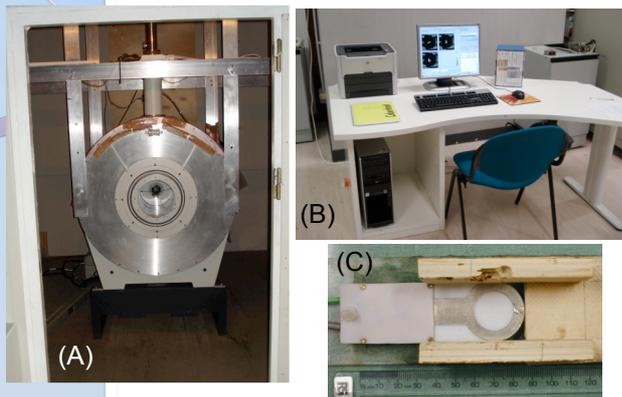
Fig. 1 (A) 2.35 T superconducting Bruker magnet (25 cm free bore). (B) Paravision 4.0 console. (C) Proton receive-only RF surface coil (20 mm diameter).
