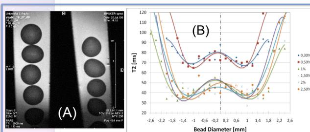
Fig. 3 (A) Coronal RARE images (TR=15s; TE=50 ms) of alginate beads at 2.5% (left) and 2% (right). (B) T2 relaxation time along the bead diameter for various initial alginate concentrations (0.3-2.5%).
