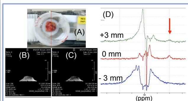
Fig. 5. (A) Human GBM tissue sample ready for high-resolution MRI; Axial MSME images (TR=6s; thickness =1mm) obtained at TE=40 ms (B) and TE=90 ms (C); (D) Water suppressed PRESS spectra (TR=6s, TE=20 ms) from a cubic voxel (3mm) at 3 different positions within the tissue. The lipid peak is shown by the arrow.
