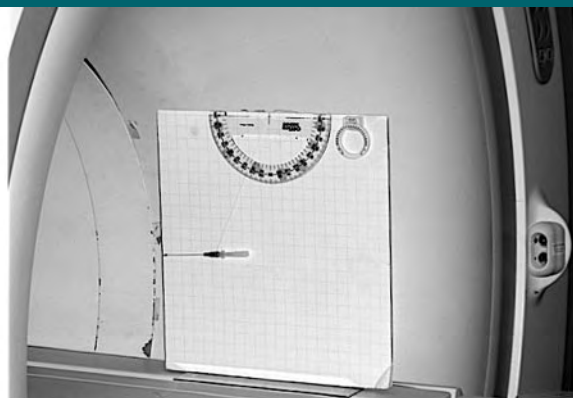
Figure 3: Example of the position of the highest spatial magnetic gradient (720 G/cm for the 3-T MR system used for testing in this case) used for the deflection angle measurement performed for an intravenous catheter. This point was inside and near the inner part of the bore of the MR system. Note the deflection angle of 24°.
